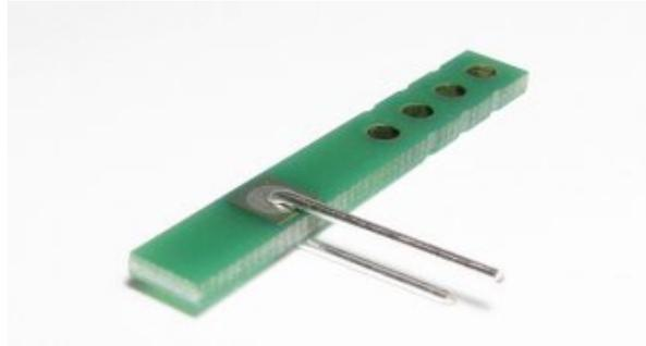
The wire must be soldered to the contacts of the board on both sides. Then it has to be put through the boreholes of the main circuit board:
