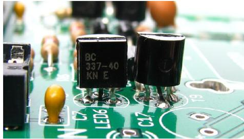
**!! Important !!** The NIBObee must never be switched on **without inserted IC3** (74HC139), otherwise the **transistors will be destroyed!**
