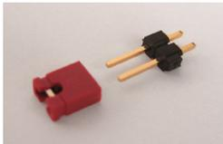
The best way to place the jumper **JP7** onto the board is to solder them complete (connector and bridge). You should pay attention to a short soldering time so that the plastics do not melt.
