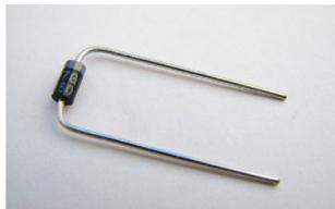
Also the Silizium diodes **D1-D8** of type 1N4007 must be bend like the resistors before placement. **You have to pay attention to the polarity:** The white line on the board print, respectively the printed
