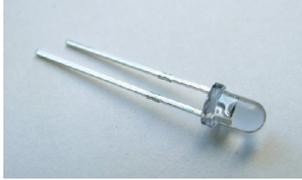
The IR-LEDs **IR3** and **IR4** have to be soldered onto the board ②.
