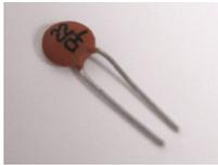
The four ceramic plate capacitors **C1**, **C2**, **C12** and **C13** have a capacity of 22 pF (imprint: 22). You don't have to pay attention to the polarity.
