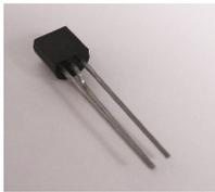
The five PNP bipolar-transistors **T1, T2, T3, T6** and **T7** are of the type BC327. During placement you have to **pay attention to the polarity!** The **flat side** of the transistor is marked on the circuit board.
