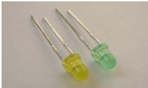
The LEDs **LED0 - LED6** have got two legs, a short one (cathode) and a long one (anode). **You have to pay attention to the polarity:** The leg with the **short length** must be placed into the **rectangular** soldering pad.
