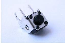
The placement of the buttons **SW1** - **SW4** is protected against polarity reversal. You have to place it onto the board with soft pressure till it snaps in. (see the picture of the finished main circuit board on page 15).
