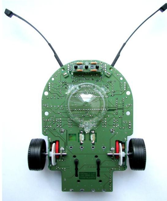
Finally the big half sphere must be put onto the NIBObee – now the robot is ready for takeoff!
