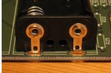
The soldering contacts of the battery packs of **type A** must point to the **middle** of the main **circuit board**.
