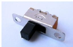
The toggle switch **S1** may be soldered onto the board in both possible orientations, the functionality stays the same.
