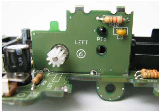
The soldering contacts of the motor have to fit exactly into the recess of the main circuit board:
