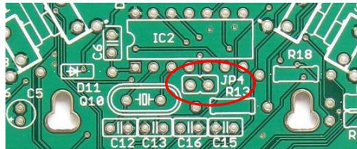
**3. Four additional data bits for the extension ports X1 and X4.**
