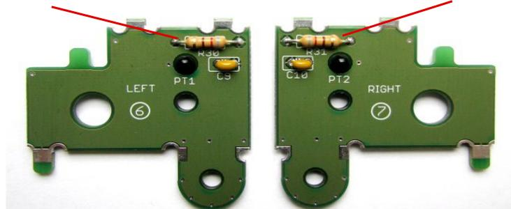
**Hint:** The resistors and the capacitors on the boards ⑥ and ⑦ have to be soldered plain onto the boards, so that they don't interfere with the driving unit in the end!
