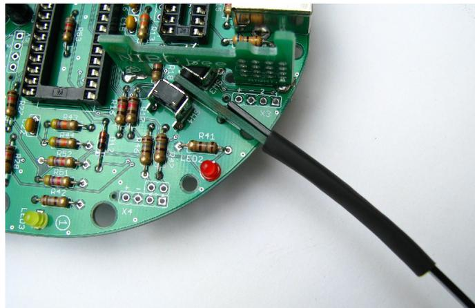
While shrinking the soldering iron should have at least 3 mm distance to the heat-shrinkable tubing.
