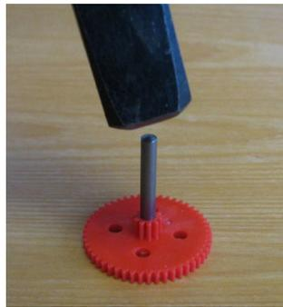
Then you have to press the axis **carefully** with the small hammer through the gear. Afterwards the gearwheel should be in the middle of the axis:
