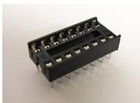
There are four IC-sockets to be soldered onto the board. The 40 pin socket is for the main controller ATmega16, the **14 pin** socket is for the ATtiny44, the **16 pin** socket is for the demultiplexer 74HC139
