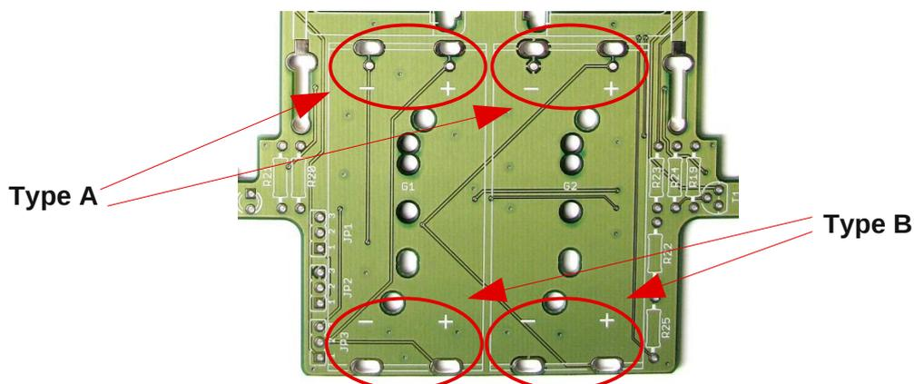
The “+/-” labels of the board and of the pack **only** has to suit at the **side with the soldering contacts**.
