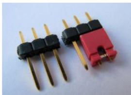
The 3-pole jumpers **JP1**, **JP2** and **JP3** have to be soldered analog to the 2-pole ones.
