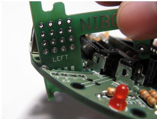
Now the board ⑥ must be pressed on from the bottom side. Therefore you hold the boards ④ and ⑤, turn the main circuit board and press the board ⑥ on so that you can see the electronic parts of the board ⑥.
