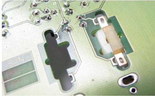
As soon as the motor fits correctly the board ⑥ is soldered to the main circuit board beginning with the middle soldering contact (see pictures).
