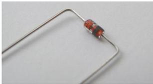
The Zener diodes **D9** and **D10** of type BZX83V003.6 (respectively 55C3V6) and the Schottky diodes **D11**, **D12** and **D14** of type BAT85 must be bend like the resistors
