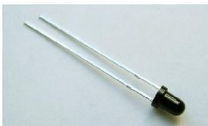
The photo-transistors **PT3-PT5** are for measuring the reflected IR-emission. They are soldered onto the board ③.
