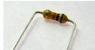
The value of the resistors is indicated by a four band colour code on the resistor, which is explained in the appendix.
