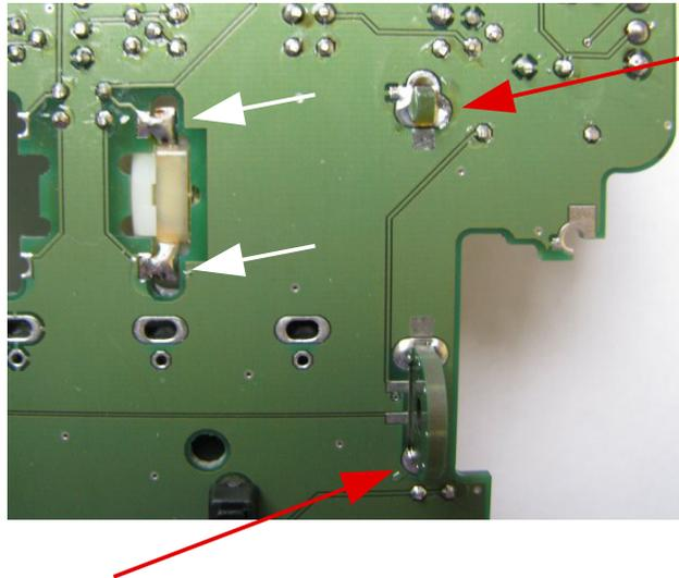
Then the motor contacts have to be soldered to the board (white arrows).
