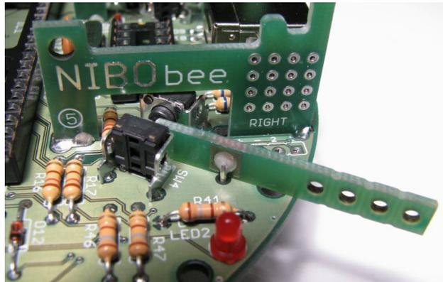
At the bottom side the wire must be fixed with the small square supporting circuit boards. First put the wire through the boards and then fix it by soldering:
