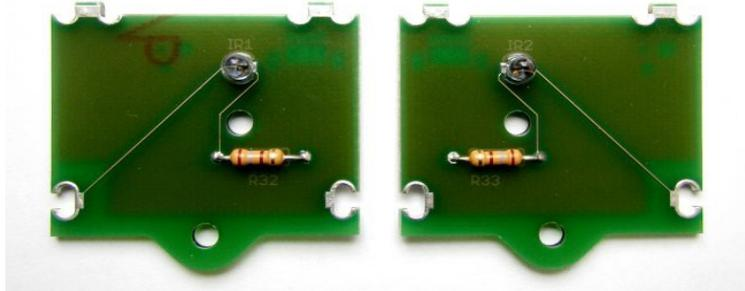
None electronic parts have to be soldered onto the boards ④ and ⑤.
