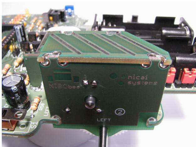
From the outside the boards have to be soldered at four points:
