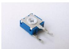
Placing the potentiometer **R29** you have to **pay attention to the polarity**: there is only one possible orientation. The potentiometer is to adjust the sensitivity of the odometry sensors.
