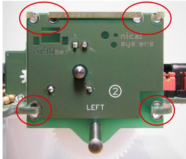
Tin the respective points **sparse** with tin-solder and heat the points afterwards about **10 seconds** with the soldering iron.
