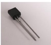
The four NPN bipolar-transistors **T4**, **T5**, **T8** and **T9** are of the type BC337. During placement you have to **pay attention to the polarity!** The **flat side** of the transistor is marked on the circuit board.
