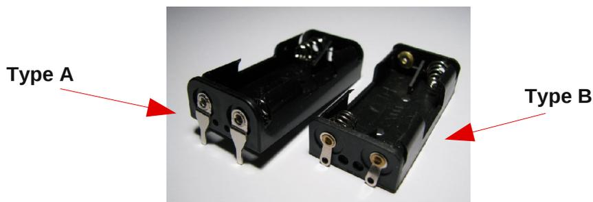
**Before assembling** the packs you have to pay attention to the “+/-” labels on the circuit board and to the “+/-” labels of the respective battery pack (the important side is the **side with the soldering contacts**: the outside contact plates).
