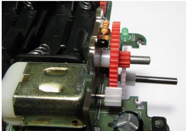
The transmission is fixed by the board ② (the electronic parts of the board ② point inwards). Finally the covering plate is pressed onto the boards ⑥ and ② with careful pressure (see image).
