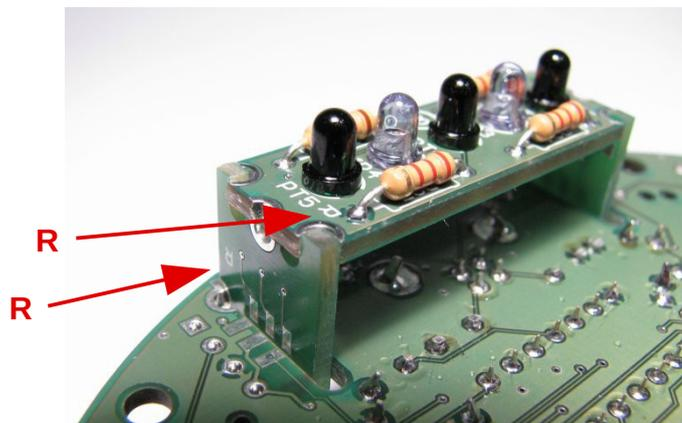
If everything is **well aligned**, the boards are now fixed by soldering. First of all just the both **middle placed** soldering points of the board ⑧ are soldered (red arrows). Then the boards ④ and ⑤ are soldered with the main circuit board (white arrows).
