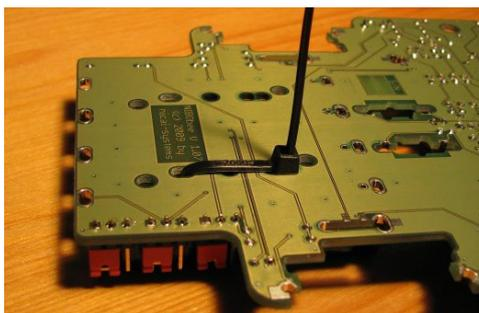
The cable strap has to be cut shortly with an electronic cutting pliers.
